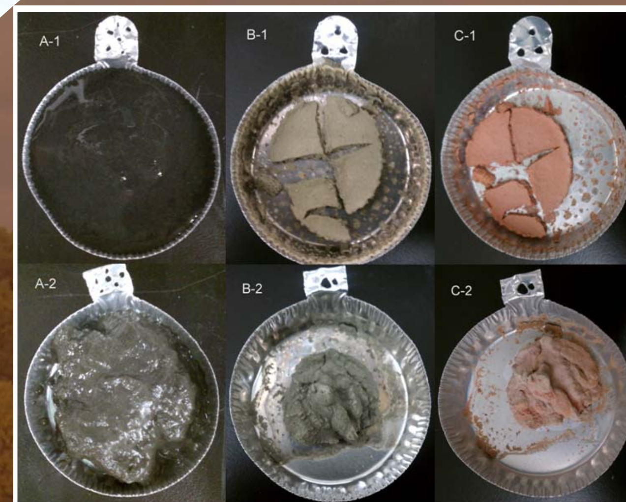
Figure 2: Top vs. bottom sediment layer changes during loss on ignition analyses. A) wet sample B) sample dried at 80 °C overnight C) sample ignited to 550 °C for 4 hours.
