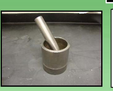
1. Cutting and Pulverization \*Samples will be cut to a desired mass using a rock saw, then crushed into fine powder using a steel mortar and pestle
