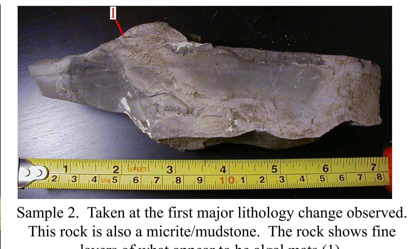
Sample 2. Taken at the first major lithology change observed. This rock is also a micrite/mudstone. The rock shows fine layers of what appear to be algal mats (1).
