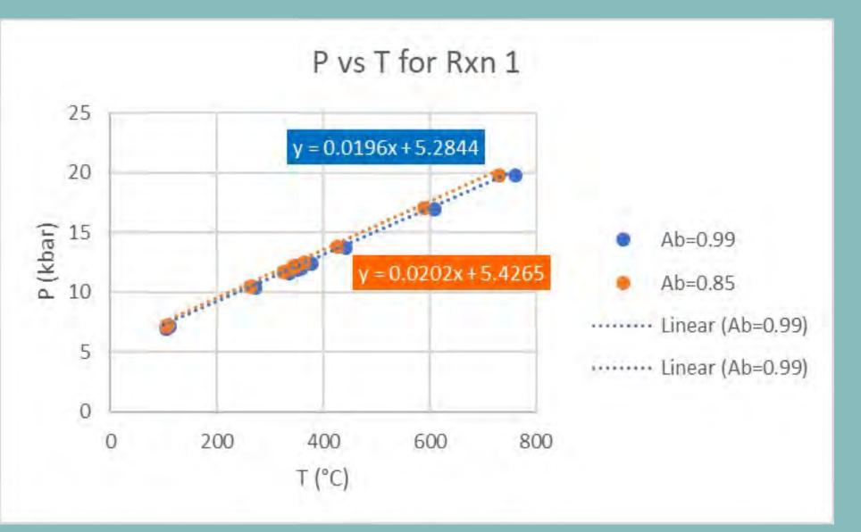
Figure 5: This graph displays the equilibrium pressure-temperature conditions calculated using the TWQ database using the range of plagioclase compositions (X<sub>Ab</sub>) present in the rock. Jadeite is stable above the lines of equilibrium while albite is stable below them.
