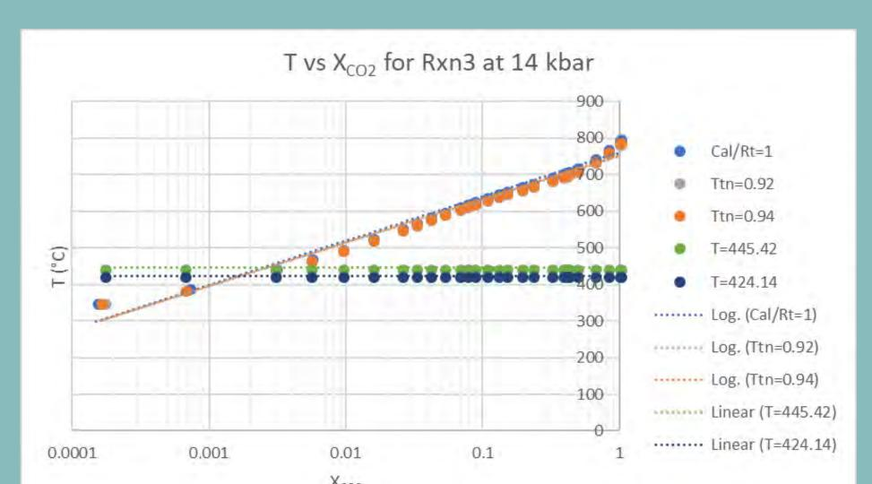
Figure 7:: The horizontal lines represent the stability of reaction 1, the inclined lines represent the stability of reaction 3. The intersection of these line sets represents the required fluid composition for metamorphism.  $X_{CO2} = 0.0025$
