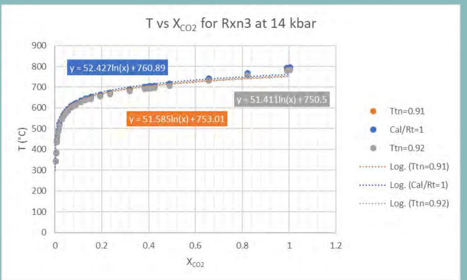
Figure 6: This graph displays the line of equilibrium above which, titanite and CO<sub>2</sub> are stable and below which, rutile, quartz and calcite are stable.
