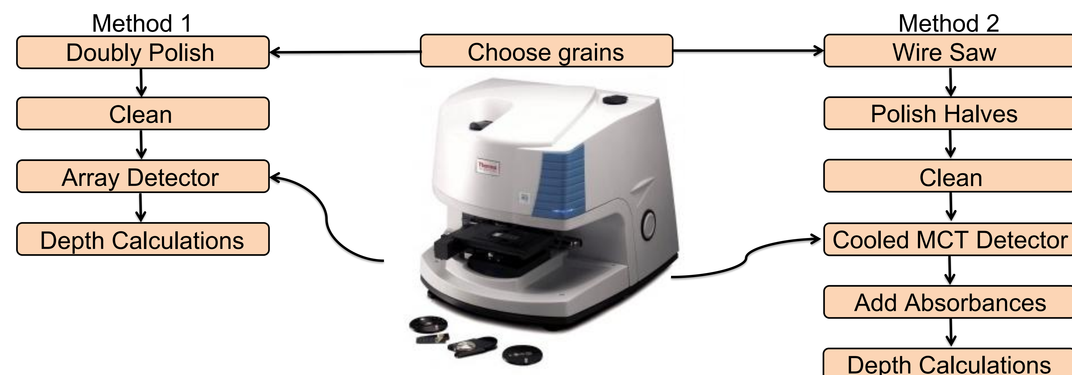
Fig. 1: A step-by step representation of the methods from choosing a grain, cutting it in half, polishing it, analysis, and calculations that yield the depth for each sample.
