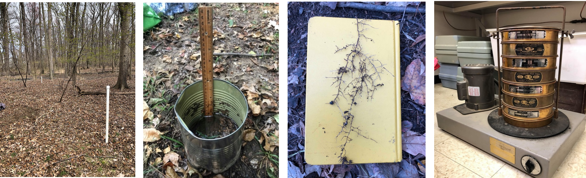
Fig.2: (left) View of the floodplain site with one of the water wells. (left center) Single-ring infiltration ring. (right center) A root from the floodplain site. (right) Mechanical shaker for sieve grain size analysis.
