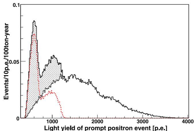
**Fig. 2.** Expected prompt positron event spectrum as obtained from the MC code, using the distribution in Fig. 1 as input and the selection cuts described in the text. The horizontal axis shows the number of p.e. detected by the PMTs. Primaries generated are  $10^5$  events for both geo- $\bar{\nu}_e$  and reactor- $\bar{\nu}_e$ . See text for details.
